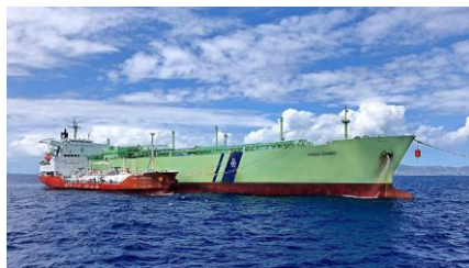
Gas vessel conducting ship-to-ship transfer. Photo courtesy of Epic Gas
