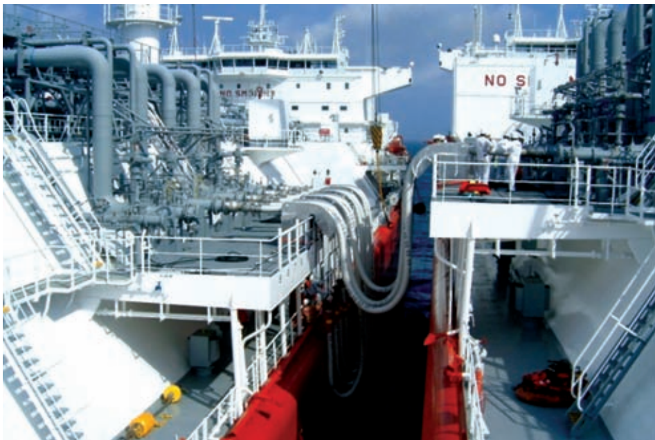
Two Exmar LNG vessels performing a ship to ship transfer – off-hire of these vessels is unacceptable for the company
