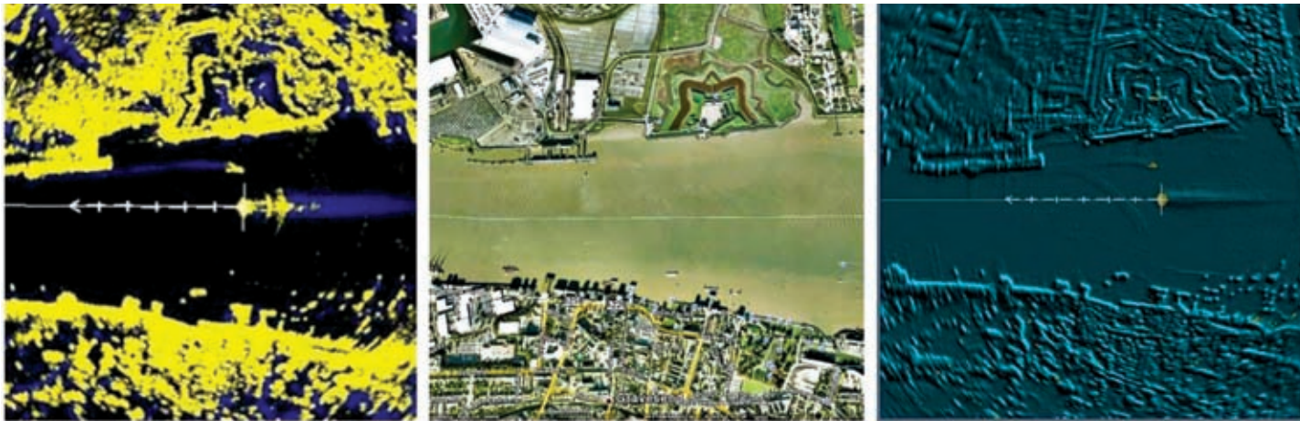
The normal radar image (left) and satellite image (centre) are combined in the enhanced display mode (right)
