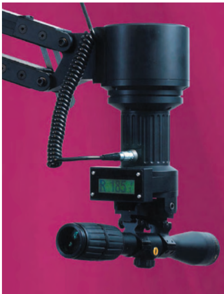
The SR02-01 can hold up to 99 bearing observations at a time
