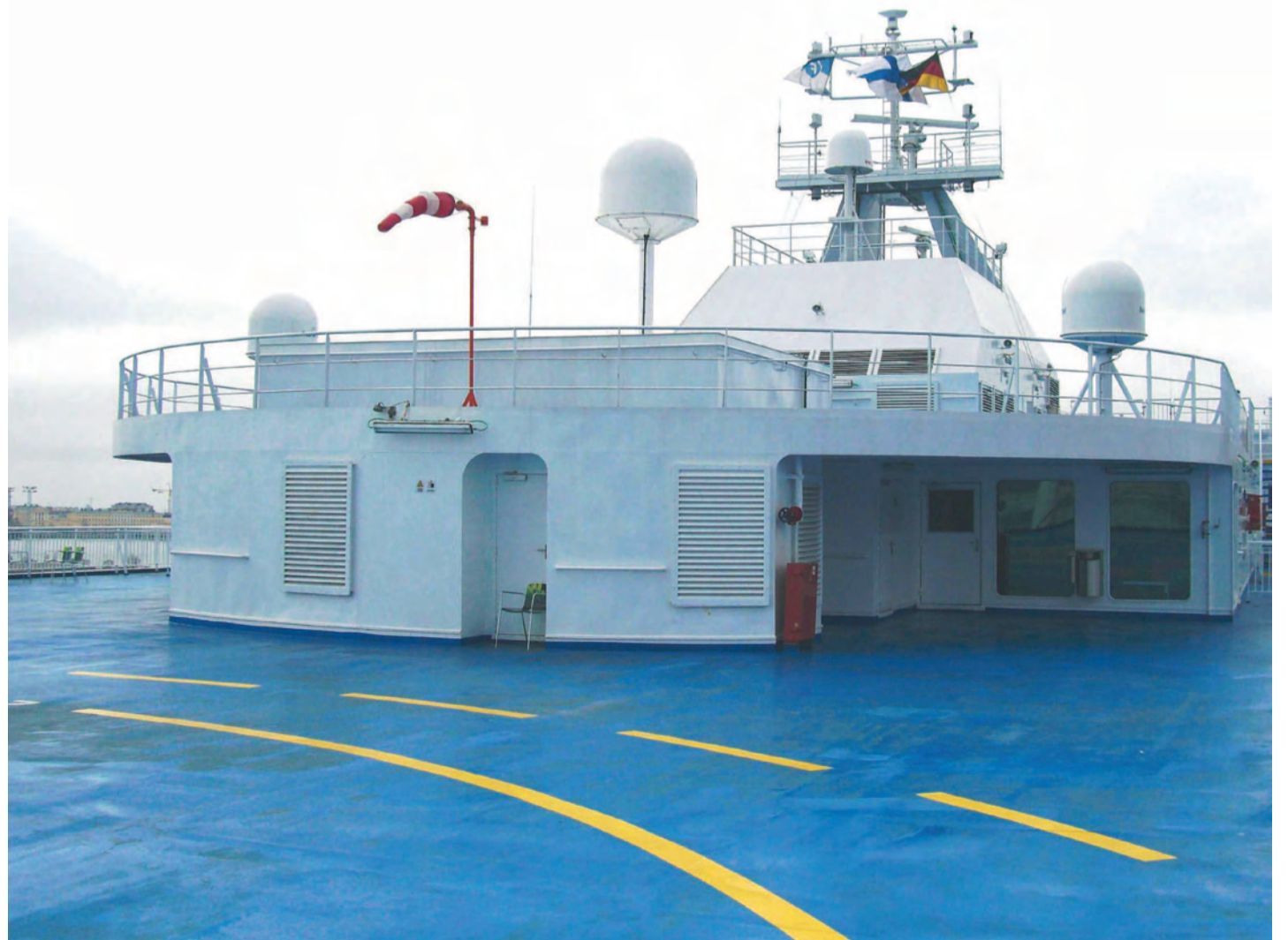
Finlines vessels carry two television antennas, installed on either side, with a 1 metre Ku-band VSAT in the middle and a Fleet 77 as back-up
