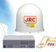
JUE-410F Inmarsat Fleet F77 Mobile Earth Station
