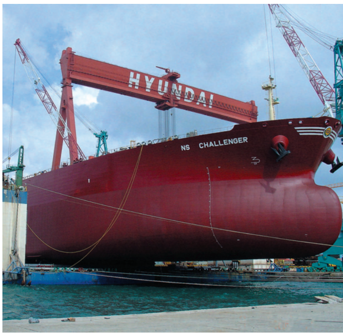
The Aframax NS Challenger was built on dry land and was launched by semi-sub barge.
