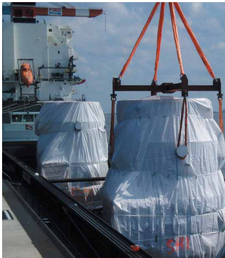
Korean shipbuilders are trying to move away from importing European manufactured high tech equipment. Seen here are the world's largest gas combustion units manufactured by Saacke. They were shipped from Bremerhaven to South Korea to be fitted on a Q-Max LNGC building at Samsung for delivery next year.
