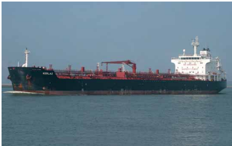
The 2004-built Kerlaz seen arriving at Rotterdam. She is a classic example of a Hyundai Mipo 37,000 dwt tanker and is operated by French concern SOCATRA.
