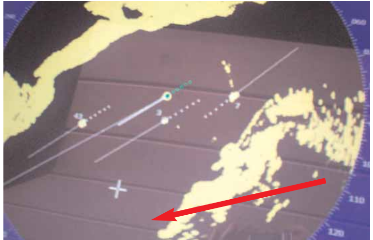
As plotted on radar screen at Nara Point. No 3 target is the overtaking vessel. No 7 target is the Northbound bulk carrier. No 43 is another southbound tanker. The start of the turn is highlighted by the arrow.
